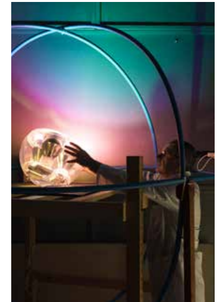
EMC Test - Triple Loop Antenna
