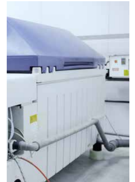
Corrosion Test - Salt-acetic fog chamber
