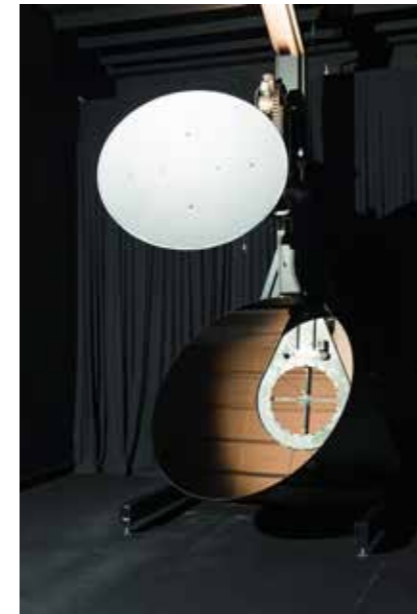
Photometric Measurements - Goniophotometer with rotating mirror
