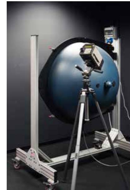
Photometric Measurements - Ulbright Sphere
